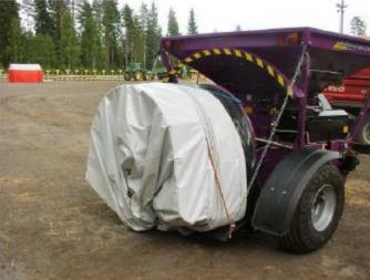
5. The tube should be made on an even and compact surface. Start making the tube against a wall, round bale or similar support. After filling about 1–2 metres, the weight of the bag is enough to keep it from sliding backwards.
