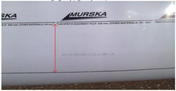
For example:  $\emptyset$ 1.5m of bag will hold c. 1.7 tonnes of grain per meter. If the crimping rate is 30 tonnes/hour, the bagger must move c. 30/1.7m/h = 17m/h = 30cm/min.
