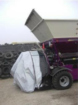
3. Pull the bag out 2–3cm holding on to the lowest fold. Make sure that the bag also unfolds evenly on top of the bottom plate and that only one layer is unfolded at a time.
